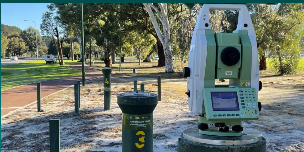
EDM Baseline located at Curtin University - one of three EDM calibration facilities in WA maintained by Landgate.
